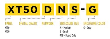
Note: Models ending in PCB indicate it is the PC board only, no cabinet. Unless sold in a kit or package, the XT panel does not include a power supply and the 321 power supply must be ordered separately.
