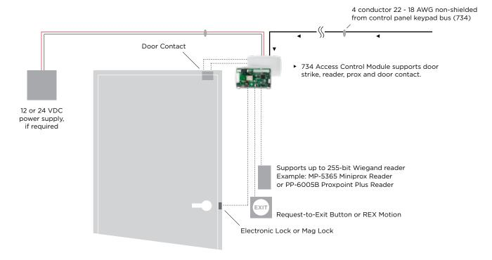
Unlike the access control capabilities of our XR Series™ panels, the door access capabilities of the XT panel are basic. The biggest advantage of XT50 door access is the ability to easily grant access to doors electronically. Concerns of unreturned keys and key duplication are eliminated by using this functionality. On the XT50 panel, all enrolled cards will work on all system readers at all times.
