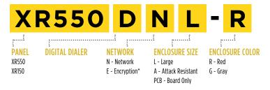
\*Encryption only available on XR550 panels. Note: Models ending in PCB indicate it is the PC board and power supply only, no cabinet.
