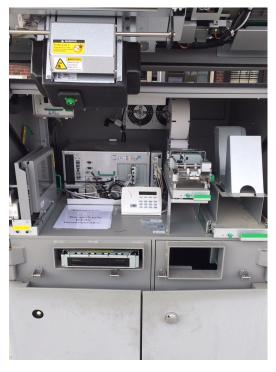
Switching out the ATMs' master key cylinders is a good preventative. Combining that with a keypad is even better. To disarm the system with the keypad, technicians can each have a unique user code. They could also use a prox card with their authorized credentials.
