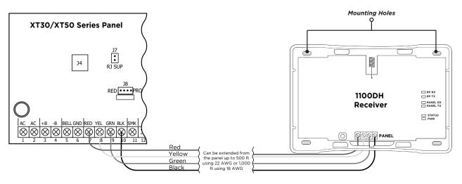
Figure 2: Wiring the 1100DH to the Panel
