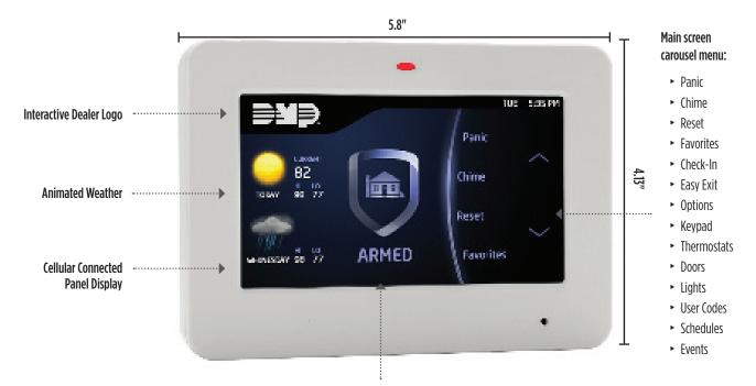
**Arming:** Tapping the shield displays an arming options screen.
