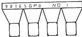
The last statement on the display, "NO 1" is telling you that the code number has been placed in the first position. The **SECURITY COMMAND** will clear the above message and request your level eight code again. The **SECURITY COMMAND** will request your code number following the addition or deletion of each code number. If no number is entered in 5 seconds, the feature will terminate.
