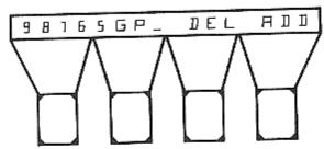
The **SECURITY COMMAND** is requesting what group number the code is to have. This feature does not apply to residential systems, therefore, "ZERO" should be entered. The following will then be displayed:
