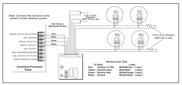
Figure 1: Panel and device connections to the 715 Loop Expander
