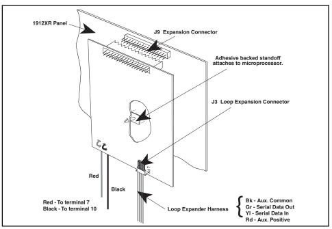
Figure 1: Installing the 881 on the 1912XR panel
