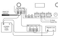
Figure 4: Magnetic Lock with an Isolation Relay
