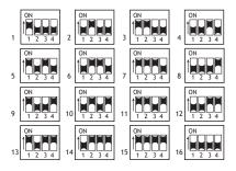
Figure 10: 734N-Wi-Fi AX-Bus Addresses
