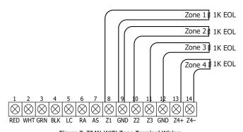
Figure 7: 734N-WIFI Zone Terminal Wiring
