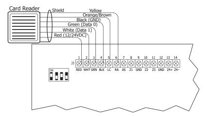
Figure 8: Card Reader Wiring
