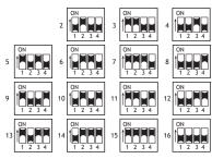
Figure 9: 734N-Wi-Fi Keypad Bus Addresses
