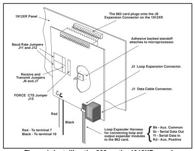
Figure 1: Installing the 862 on the 1912XR panel
