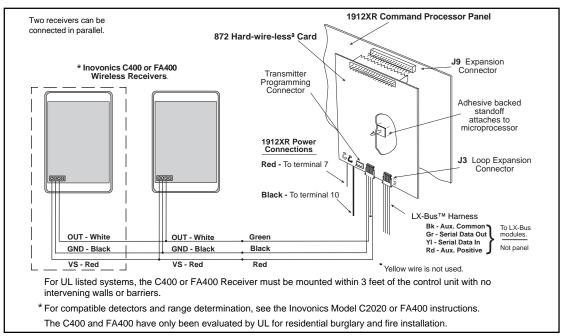
Figure 1: Wiring for the 400 series receiver(s) and 872 card.
