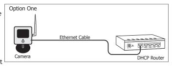
2. Once the Ethernet is plugged in, plug in the power adapter to the camera, and to a power outlet. The Power LED, which is located on the front of the camera, just above the PIR detector, turns solid for 20 seconds while powering up. When the camera is fully powered on and finds an active network, the power LED begins to flash green.
