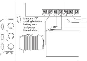
Figure 6: Transformer Installation
