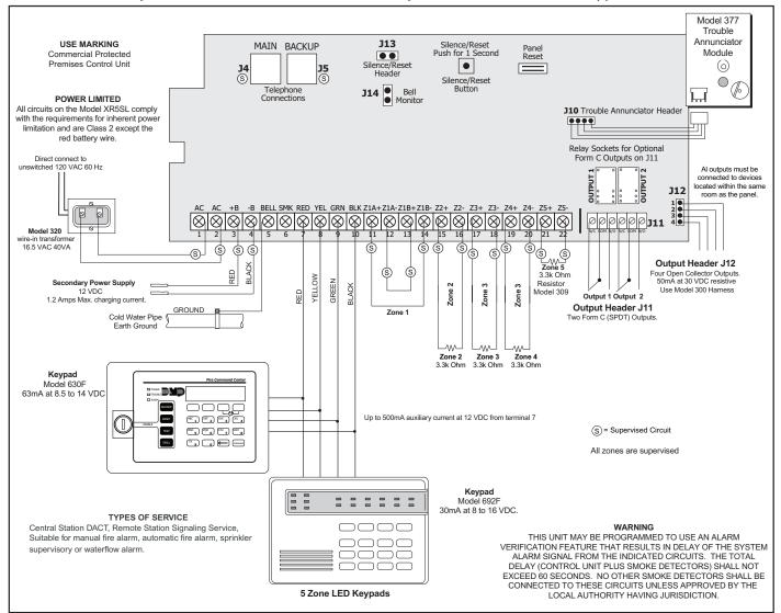
Figure 2: XR5SL Wiring Diagram
