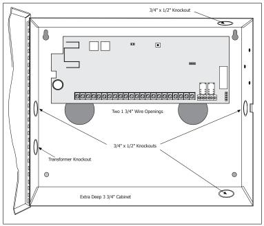
Figure 3: Mounting the Enclosure
