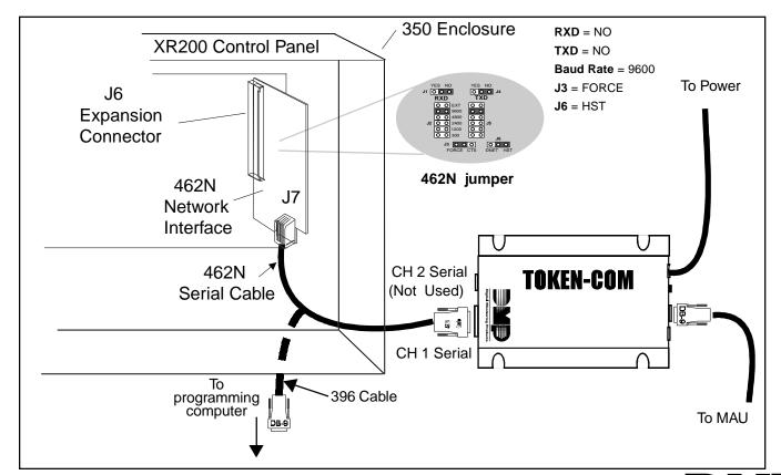
Figure 1: Token-Com Installation
