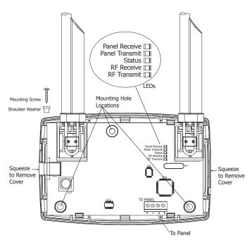
Figure 1: Receiver PCB
