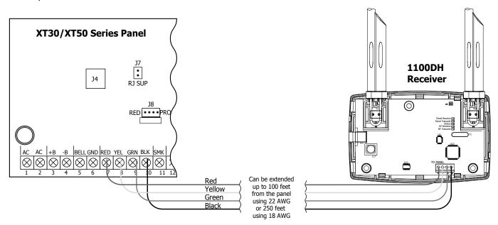
Figure 2: Panel Keypad Bus Connection
