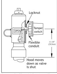
Figure 5: Clow Valve Installation
