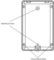
Figure 3: Mounting Holes
