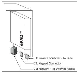
Figure 1: ePAD 3-Hole Pattern Installation
