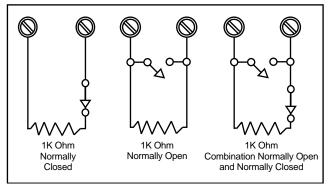
Figure 14: Protection Zone Wiring
