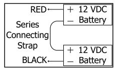
Figure 4: 24 VDC Battery Wiring
