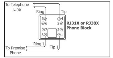
Figure 7: Phone Jack Wiring
