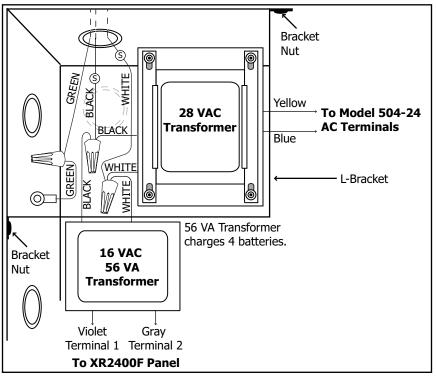
Figure 3: Transformers and AC Power Connection
