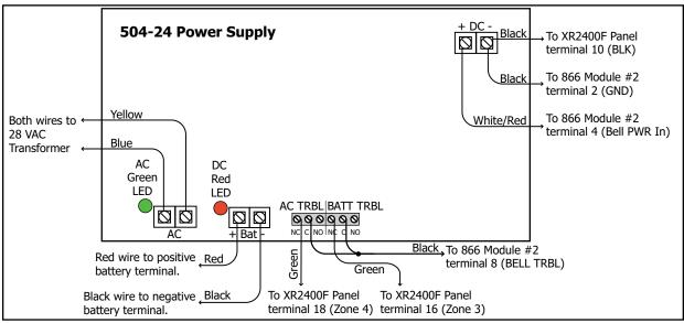
Figure 9: 504-24 Wiring
