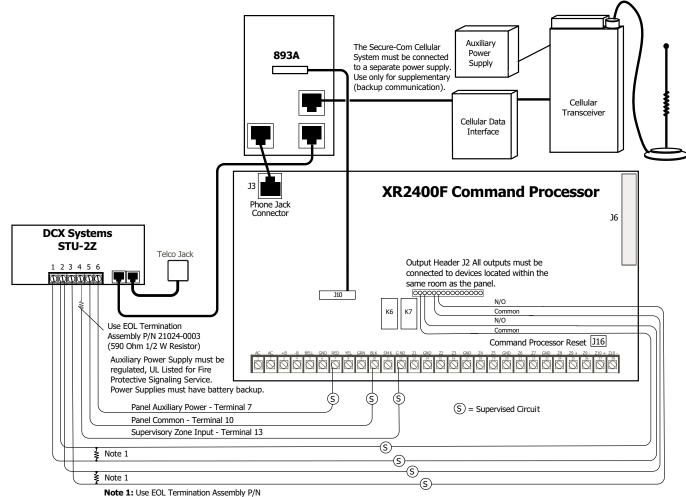
Note 1: Use EOL Termination Assembly P/N 21024-0001 (2.2k Ohm 1/2 W Resistor).
