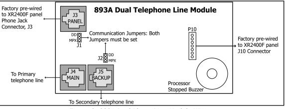
Figure 8: 893A Dual Phone Line Module Wiring
