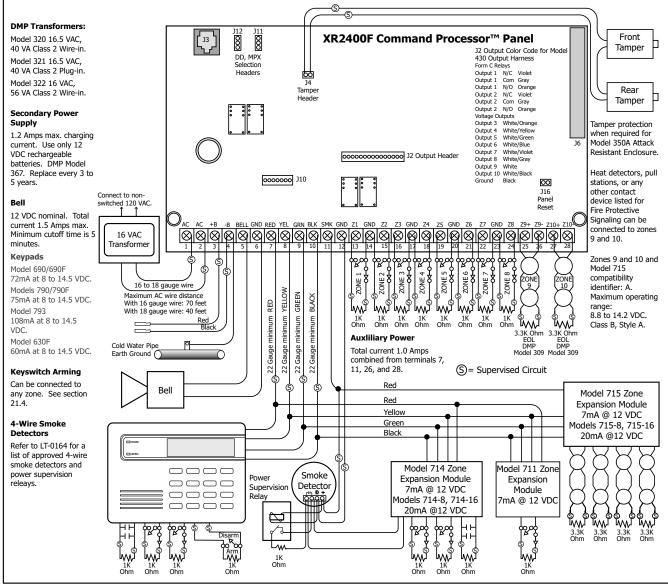
Figure 13: Typical XR2400F Wiring Diagram
