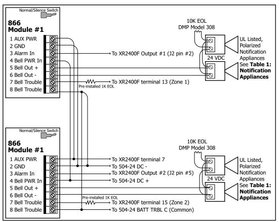
Figure 5: 866 Modules Wiring
