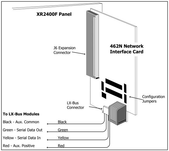
Figure 6: 462N Wiring
