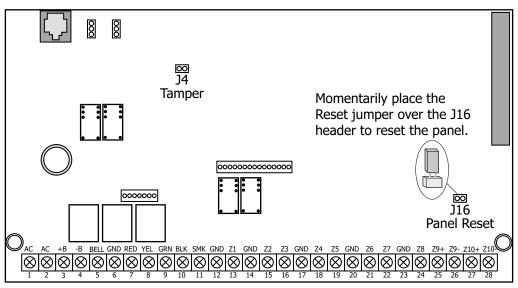
Figure 15: XR2400F Panel Showing Reset
