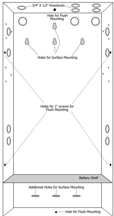
Figure 1: Mounting the XR2400F Enclosure
