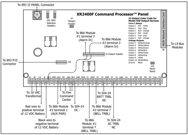
Figure 11: XR2400F Panel Wiring
