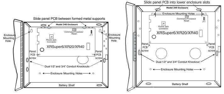
Figure 2: Standard 340 Enclosure (left) or Optional 349 Enclosure (right)
