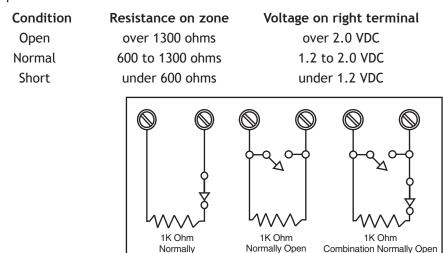
Figure 5: Protection Zone Contact Wiring
