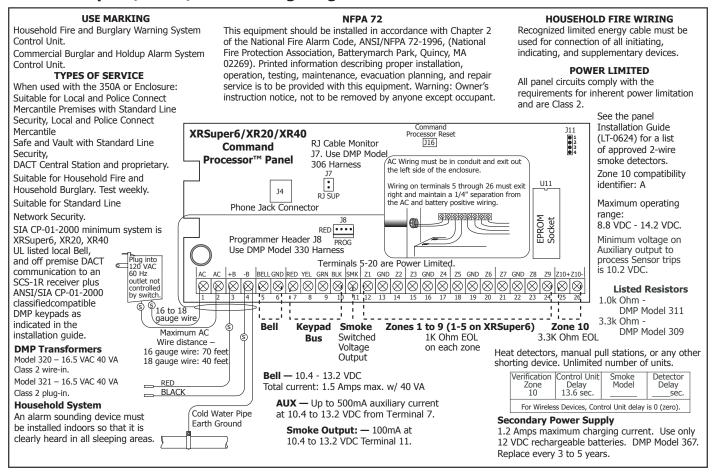
Figure 1: System Wiring Diagram
