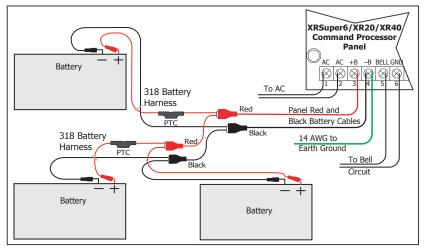
Figure 4: Wiring Multiple Batteries
