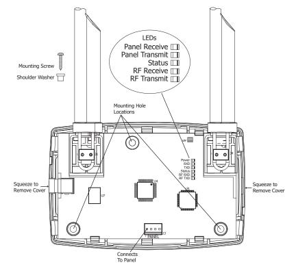
Figure 1: Receiver PCB
