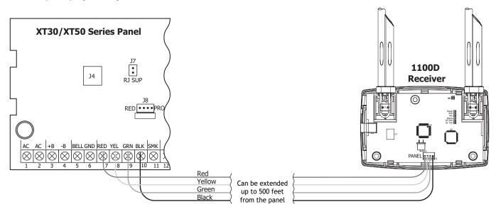
Figure 2: XT30/XT50 Series Keypad Bus Wiring
