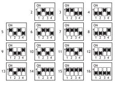
Figure 9: 734 Keypad Bus Addresses
