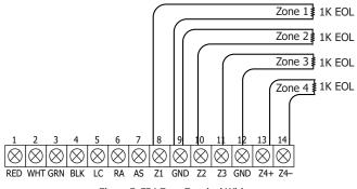
Figure 7: 734 Zone Terminal Wiring
